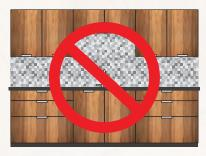
Manufacturing with tight side out construction ensures even finishing to avoid the "barber pole" effect.
