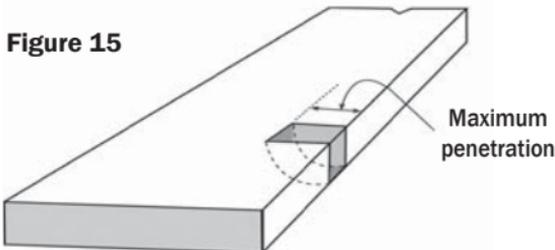
For Figure 15 saw cuts, the "**Maximum**" penetration across the width is restricted to  $\frac{1}{2}$  the allowable edge knot size.
