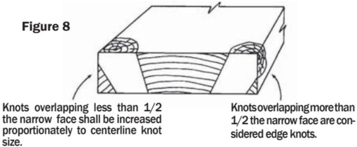
The allowable size for diagonal knots that only involve the wide face shall be proportionately increased to the size specified for knots located along the centerline (Figure 7). Diagonal knots involving both narrow faces are equated to an **Edge Knot** (Figure 9).
