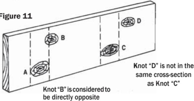
The sum of the sizes of all knots within any 6" of length shall not exceed twice the diameter of the allowable centerline knot (**Figure 12**). No two centerline knots of maximum size may appear in the same 6" of length.
