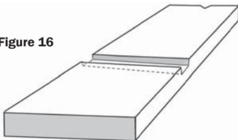
The penetration of the saw cut described in Item 2 above, as depicted by Figure 16 is restricted to  $1/2$  the equivalent edge knot displacement.
